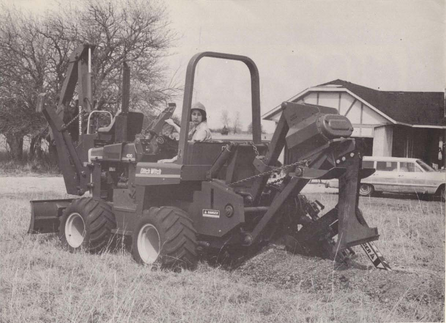
40 H.P. Class model 4010 Modularmatic which uses interchangeable modules
